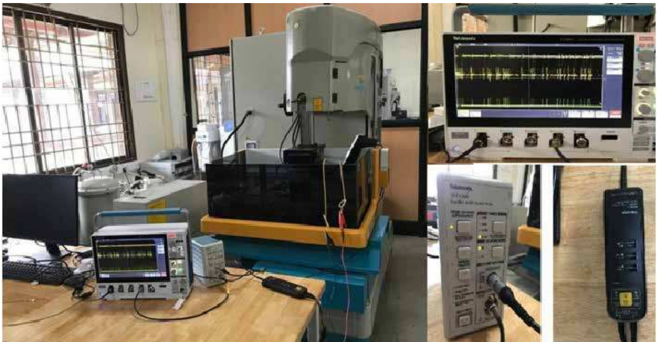
Condition monitoring setup for Wire EDM
